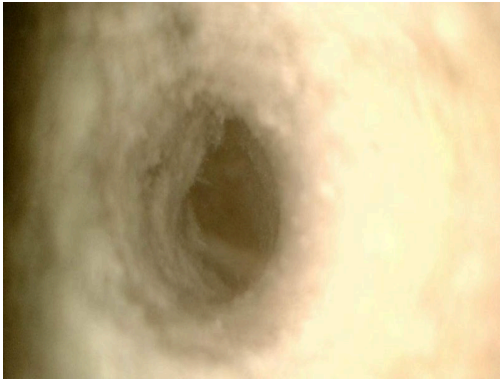
Photo indicators of filled cavity insulation:
